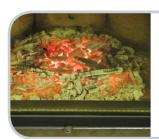
This has been achieved when the wood has been completely burnt and no smouldering fire or incomplete burn can develop. The setting lever can now be closed (left position).
